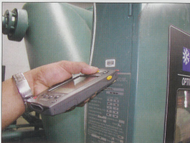
Mintek Mobile Data Solutions' WinTrack PM scanning device tracks preventive maintenance via barcodes placed on or near the equipment.
